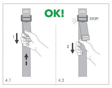
Carry out a functional check of the adjustment system for each
