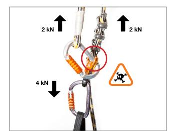
In this configuration, we have observed a failure of the rope end attachment hole of the ZIGZAG under 4 kN of charge (equivalent to short fall, repeated shock or sudden stop, etc).
