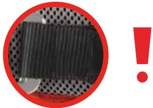
If structural sewing is missing stop use and contact DMM:
