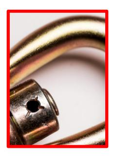
**IMPORTANT:** If you do not see the red paint or if there is no pin present or if the nut rotates or is loose the karabiner should be removed from service immediately – please return to the manufacturer in line with the corrective action at the end of this notice.
