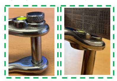
If the button is higher than the collar, the device MUST be removed from service.
