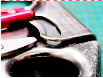
Figure 1—If there is evidence of deformation (see arrow) then you **MUST** retire the unit.
